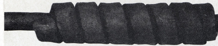
Twisted or untwisted, skelp is wound tightly around mandrel. Welding begins with “jumping up” — driving the white-hot section of barrel straight down on its end, against the face of the anvil.
